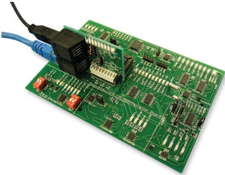
The NXP I<sup>2</sup>C-bus 2005-1 evaluation board has an available P82B96/PCA9600 daughter board to generate Fast-mode Plus signals or to drive long cable signals via two RJ45 interface jacks. Refer to application note AN10658.
