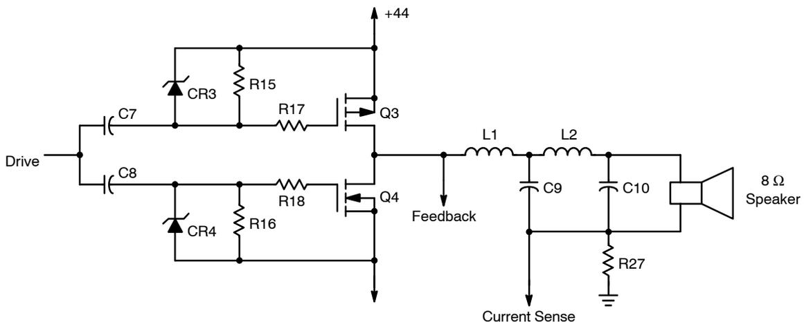
**Figure 5. Output Circuit of a Class D Amplifier**
