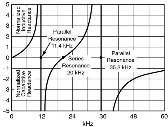
**Figure 4. Four Pole Butterworth Filter Output Impedance**
