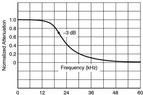
Figure 3. 20 kHz Butterworth Filter Frequency Response
