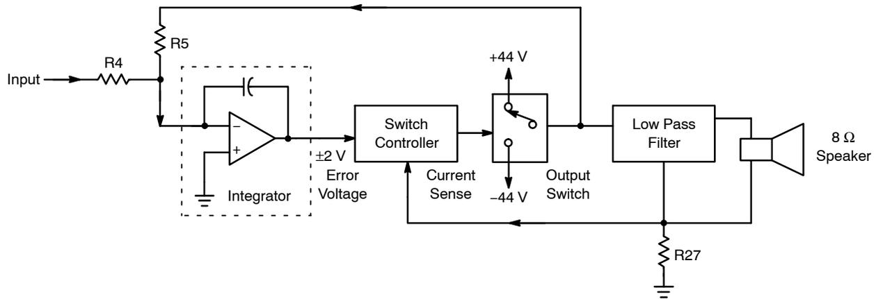
Figure 2. Block Diagram of Class D Amplifier
